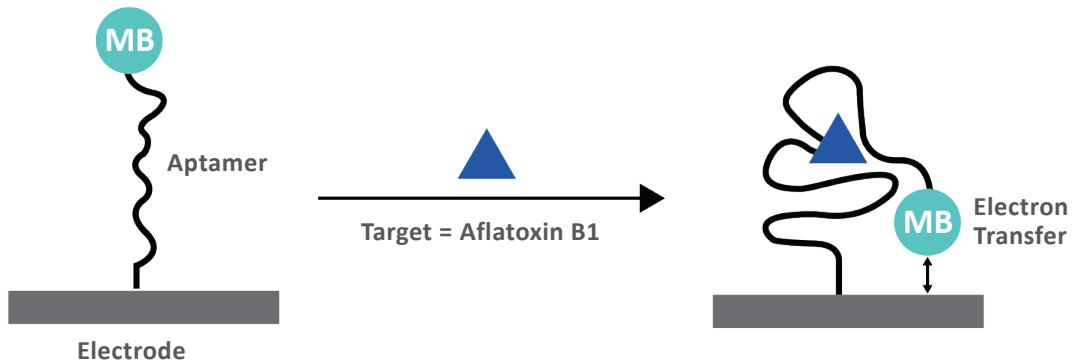
*Figure 2. Aptasensor for Aflatoxin B1 Detection*
