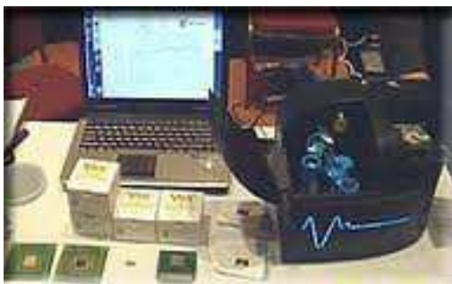
Figure 1: Vista Therapeutics Inc. NanoBioSensors™ instruments are based on detection of analytes via nanowires, microscopic wires whose conductance varies (with great sensitivity) as the concentration of target molecules passing over the wires changes. Consumable products to date include NanoCards, Functionalization Kits, and Sample Preparation Kits.
